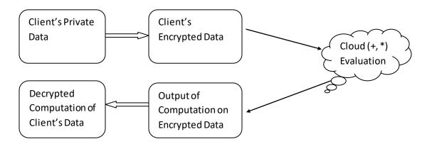
As the figure shows it utilizes bilaterally symmetric homomorphic cipher to boost data security. The client will encrypt his plain texts using a secret key generated. Then the encrypted data will be stored on Cloud Storages. If an intruder tries to hack into storage then he will find only the encrypted data. Later the client can decrypt data when needed using the same key.
